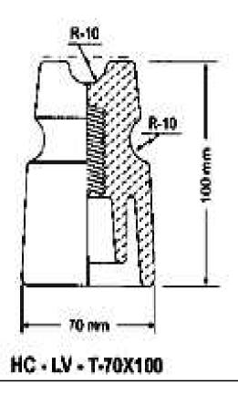
Type of Insulators Type I Standards to which insulators IS: 1445/1977 Latest will conform amendment 70 mm X 100 mm Dimensions Color of Glaze Brown Dry Power freq. Withstand 23 KV voltage (KV) Wet Power freq. Withstand 10 KV voltage (KV) Puncture Withstand Voltage 1.3 x Actual Dry Power Frequency Voltage Minimum failing Load (KN) 3.5 KN Temp Cycle test (as per ISS) As per clause 7.8 of IS 1445 Porosity test (as per ISS) As per clause 7.11 of IS 1445 Furnished drawing no. BPPL-LT-05
